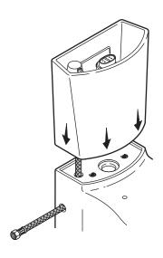
8 Slide the hose guide onto the hose, with the flared end last. Slide the two inserts into the flared end of the hose guide.
