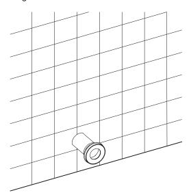
2 For floor-outlet installation, place the pipe fittings as shown
