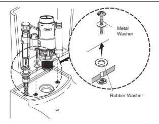
10 Thread the bolts into the bowl through the bolt holes in the bottom of the tank. Tighten the bolts using a screwdriver.
