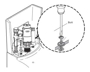
11 Carefully thread the bolts into the nuts on the brackets. Do not overtighten.
